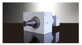
20 kHz seam welding heads, with up to 3KW power, are particularly suitable for continuous welding of tubes, solar absorbers, copper sheets... Indeed, they have been especially designed for continuous seam welding applications. These rotating heads allow producing continuous welding seams. The ultrasonic seam welding works on the same principle as the ultrasonic welding. However, the circular shape of the sonotrode coupled to a rotating mechanism enables to solder without interruption.
