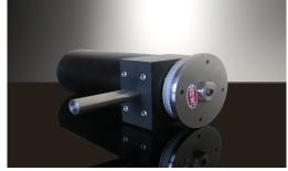
20 kHz rotating seam welding heads are particularly suitable for continuous welding of thin aluminum foil or copper foil. These rotating heads allow producing continuous welding seams, that is to say without any discontinuity. The ultrasonic seam welding works on the same principle as the ultrasonic welding. However, the circular shape of the sonotrode coupled to a rotating mechanism enables to solder without interruption.
